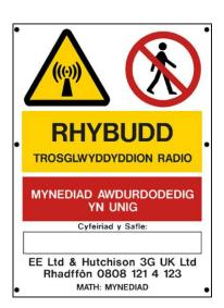
This sign will be placed at the boundary of a non-compliance area (exclusion zone). It is designed to give a clear warning of the hazard and details of the owner of the equipment.
